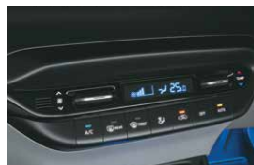
Fully automatic temperature control (FATC)
