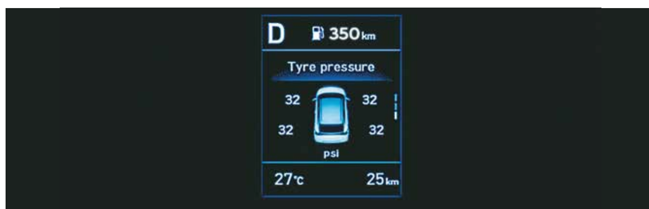
Tyre pressure monitoring system (highline) with display on MID
