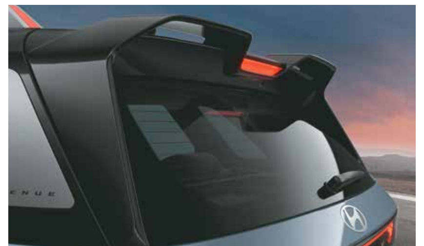
Wing type spoiler with LED high mounted stop lamp (HMSL)
